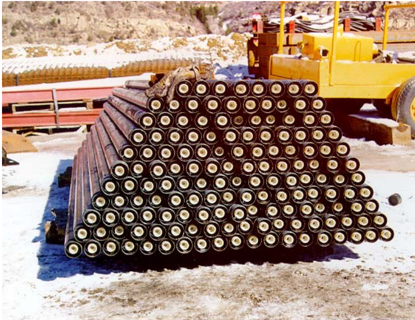
Figure 2. REI Drilling, Inc.'s high performance drill rod with streamlined DDM MECCA inserts.
