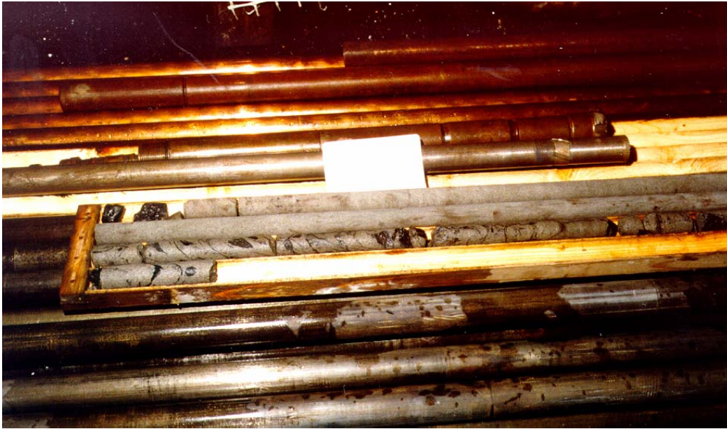
Figure 8. Cores of coal and roof contact retrieved by REI Drilling, Inc. in advance of mining at Cape Breton Development Corporation Mines in Nova Scotia, Canada.
