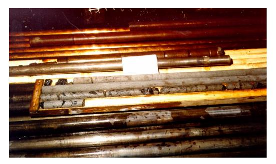
Figure 8. Cores of coal and roof contact retrieved by REI Drilling, Inc. in advance of mining at Cape Breton Development Corporation Mines in Nova Scotia, Canada.
