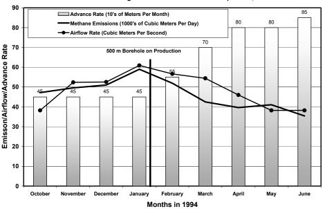
Methane Emissions, Airflow Requirements, and Advance Rate Before and After Degasification for 2 West Developments, Mine I
