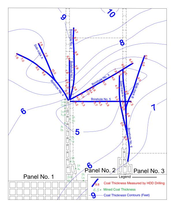
**Figure No. 1:** Plan view illustrating extent of coal thinning associated with post-depositional channeling as determined by HDD drilling to determine seam height. The anomaly affected three (3) longwall panels as indicated by the seam heights determined from drilling and the resulting isopachs.
