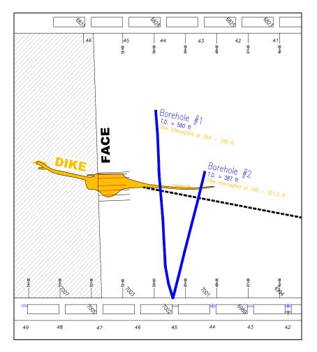
**Figure No. 6:** Plan view illustrating the directional drilling effort performed to characterize the extent of the igneous intrusion inby the longwall face. Note that face drilling indicated the dike was massive and extended inby.
