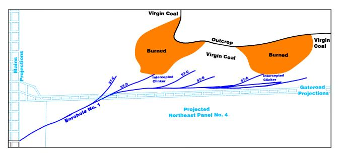
**Figure No. 5:** Plan view illustrating the directional drilling effort performed to characterize the extent of burn into the reserve. Note the exploration side-tracks developed from the main borehole to define the distance between competent coal, as verified by the main borehole, to the burn.
